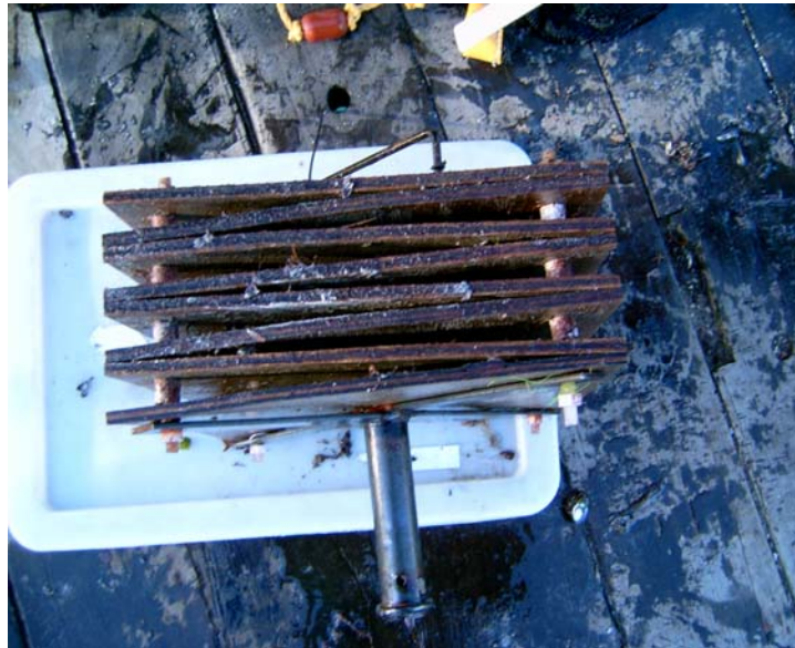
Figure 54. A crevice collector as used in South Australia, Victoria and Tasmania for puerulus settlement.
