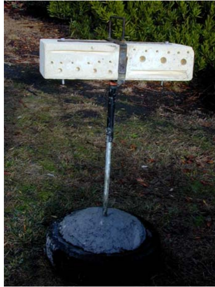
Figure 28. Hebel collector. Puerulus settled upon collectors of this design constructed of Hebel in preference to limestone.
